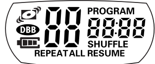
test pattern 1 (all segments activated)
